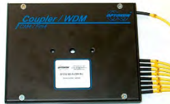
CM4 box with cable outputs
