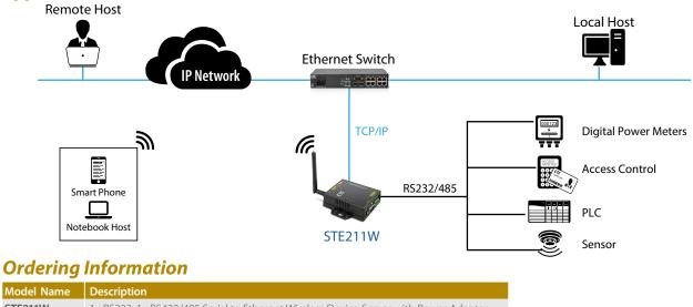
1x RS232, 1x RS422/485 Serial to Ethernet Wireless Device Server with Power Adapter STE211W **STE211** 1x RS232, 1x RS422/485 Serial to Ethernet Device Server with Power Adapter
